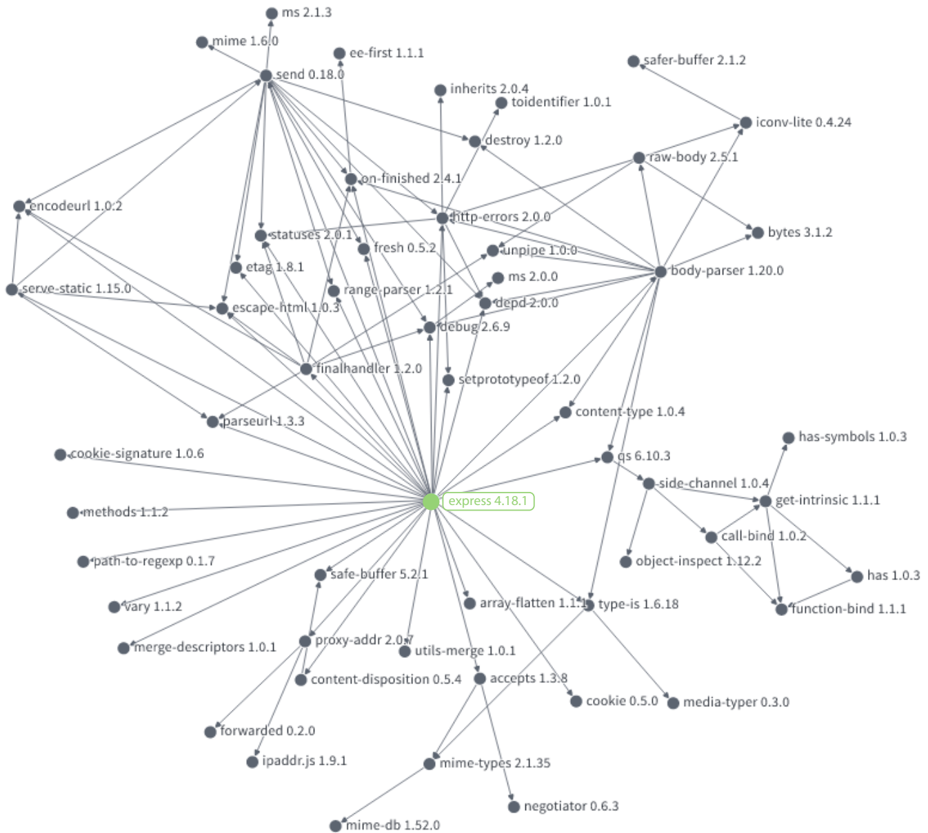
Figure 1: A dependency graph showing the names and version numbers of all direct and transitive dependencies for 'express', a popular javascript framework used to build web applications. Source: Open Source Insights
