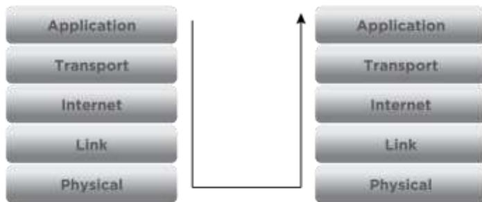
Figure **ERROR! NO SEQUENCE SPECIFIED.** – The picture above shows the reverse workflow when the message has to be reconstructed and delivered.
