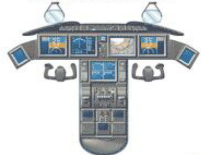
Main instrument panel, shroud and centre console
